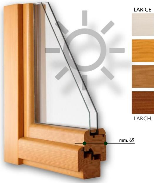
$U_w = 1.12 \text{ W}/(\text{m}^2 \cdot \text{K})$  con vetrocamera/avec vitrage isolant  $\Psi = 0.041 \text{ W}/(\text{m} \cdot \text{K})$   $U_g = 0.8 \text{ W}/\text{m}^2\text{K}$  F2 ante/volets Lm 154x148
